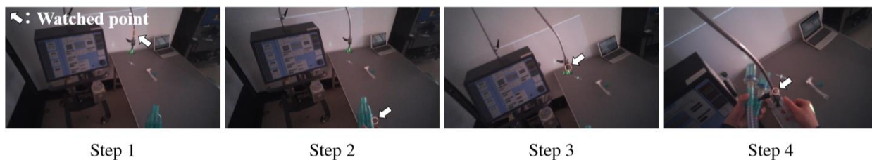
Fig.11 Movement of watched points with remote work support using projection technique
